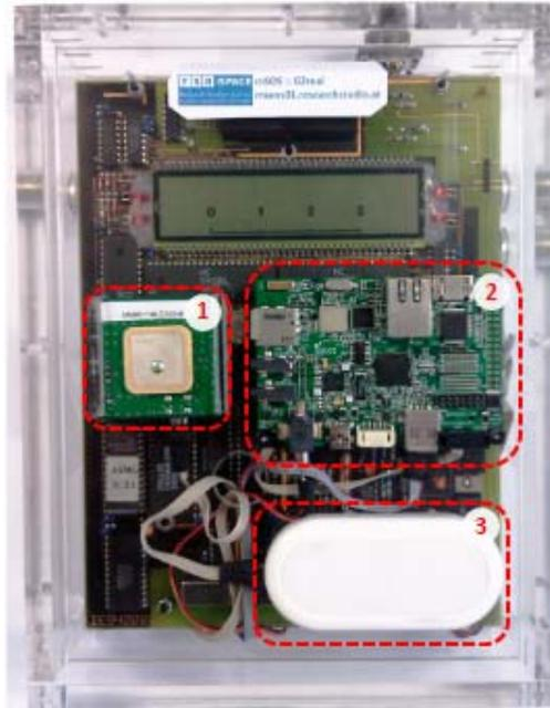
Notes: (1) GPS receiver, (2) IGEPV2 single board computer, and (3) UMTS modem on top of SSM-1 (circuit board only).
